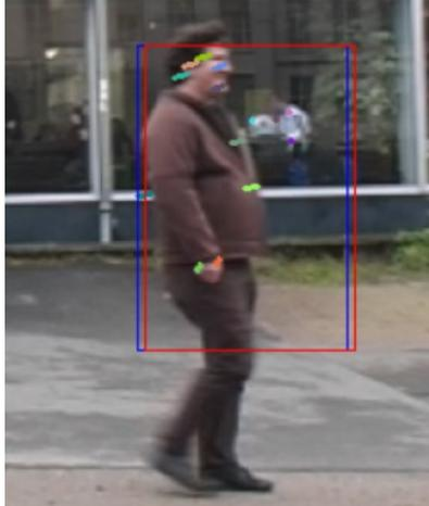
Figure 8: Example of the displacement of points between two frames, as well as the previous and next bounding boxes
